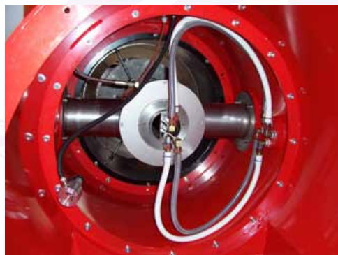
Stainless steel FGR connections inside burner
